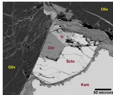
Figure 1. Reversely-zoned chromite in Sericho.
