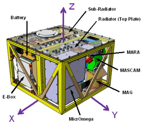
**Figure 1: Accommodation of subsystems and payloads of the MASCOT lander. Note: Radiators and closing foils on sides +X, -X, +Y, -Y -Z are not shown**
