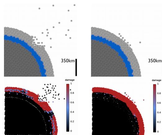
**Figure 3.** Top panel: crater-forming impact snapshots with subsurface ocean (blue) underneath the icy crust. Bottom panel: the damage plot shows that pressure propagating throughout the ocean damages the entire crust. Left column: transient crater, right column: final crater. The impact velocity and angle are like in Fig. 2.
