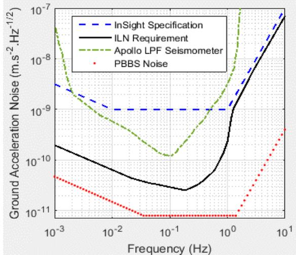
**Figure 1:** The Planetary Broadband Seismometer (PBBS) is designed to meet a sensitivity requirement necessary to achieve LGN science, as defined by International Lunar Network Science Definition Team [2].
