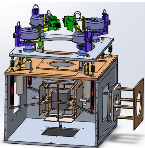
**Figure 3:** The PBBS triaxial design.
