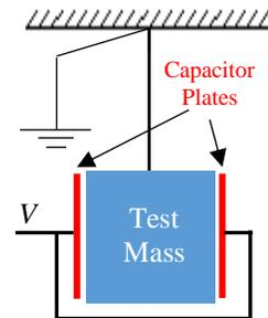
**Figure 2:** EFR counteracts the pendulum restoring force with electrostatic force.
