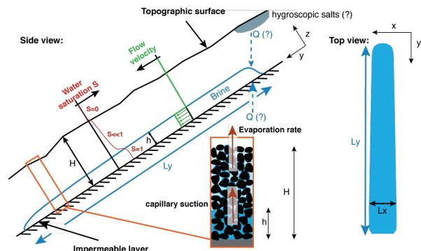
Figure 1. Schematic illustration of the wet gravity current model for RSL.
