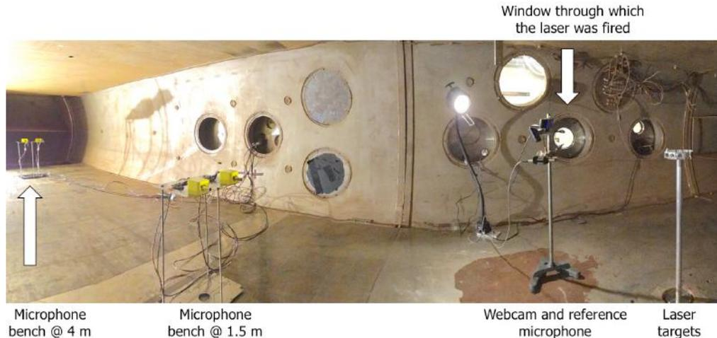
Figure 2: Panoramic photo of the test configuration inside the Aarhus wind tunnel
