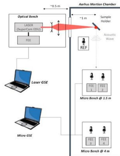
Figure 1: Schematic of the test configuration at Aarhus. FEE = Front-End Electronics; EDU = Engineering Development Unit; GSE = Ground Support Equipment.
