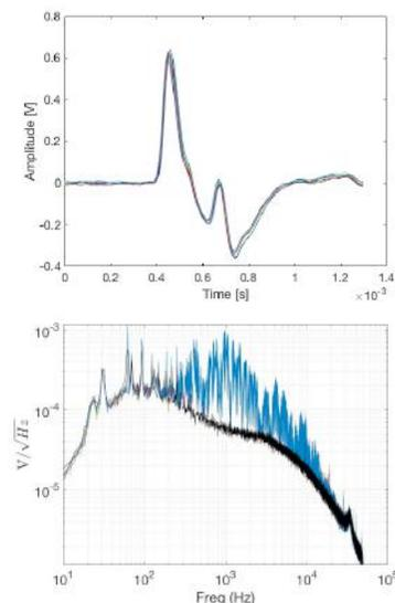
Figure 3. (Top) The waveform of a typical acoustic recording of the LIBS impact. Each line corresponds to a different laser shot. (Bottom) Typical spectra from a full 10 second acquisition containing  $\sim 50$  LIBS shots. Each spectrum corresponds to a different acquisition. The background noise in  $\text{CO}_2$  is indicated in black. All data are from tests performed in 6 mbar of  $\text{CO}_2$  and measured at 1.5 m from the Aluminium laser target.
