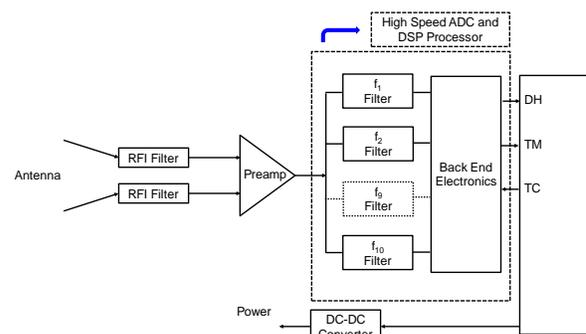
Figure 1: Preliminary design of LIVE for future orbiter
