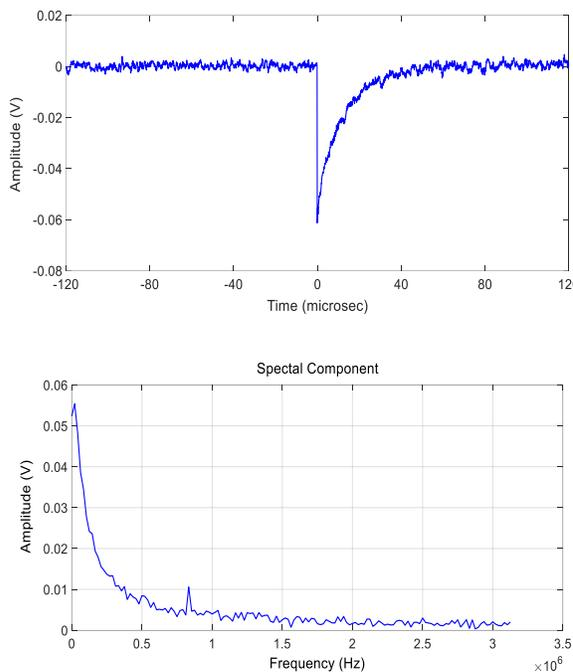
Figure 3: (a) EM pulse due to electrostatic discharge and (b) spectral components of electrostatic discharge pulse.
