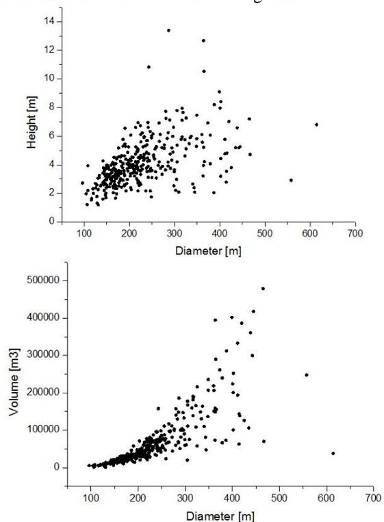
**Fig. 1** Scatter plots of diameters, heights, and volumes of the 532 RMDSs measured from NAC-derived DEMs.
