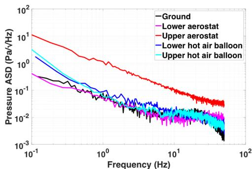
**Figure 1** (from [4]): Noise detected by barometers on various platforms. Floating platforms reduce the wind noise experienced by barometers.
