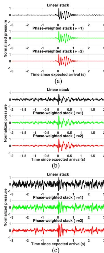
**Figure 2** (from [4]): Stacked signals from different barometers. (a) Ground barometer, (b) lower aerostat (or moored balloon) barometer, (c) upper aerostat barometer
