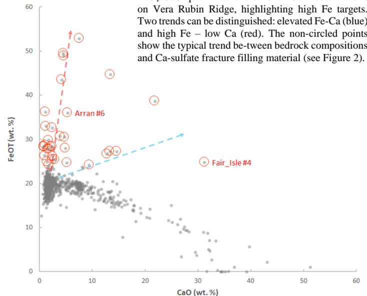
**Figure 1:** Bivariate plot showing FeO<sub>T</sub>/SiO<sub>2</sub> and FeO<sub>T</sub>/CaO quantifications of ChemCam observations on Vera Rubin Ridge, highlighting high Fe targets. Two trends can be distinguished: elevated Fe-Ca (blue) and high Fe – low Ca (red). The non-circled points show the typical trend between bedrock compositions and Ca-sulfate fracture filling material (see Figure 2).
