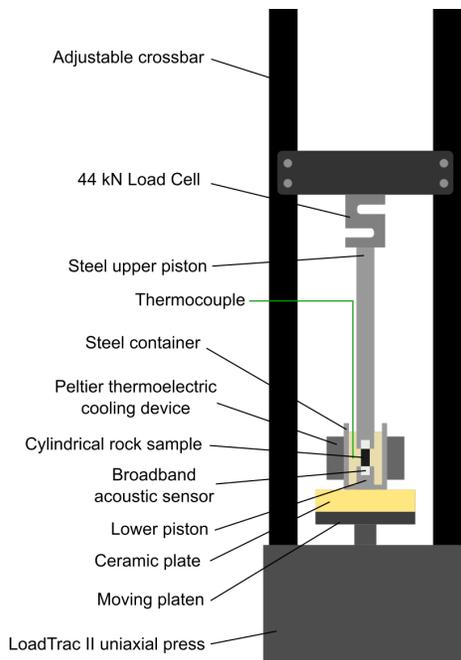
**Figure 1:** Schematic of the experimental device at the University of Strasbourg. (Illustration is not to scale.)
