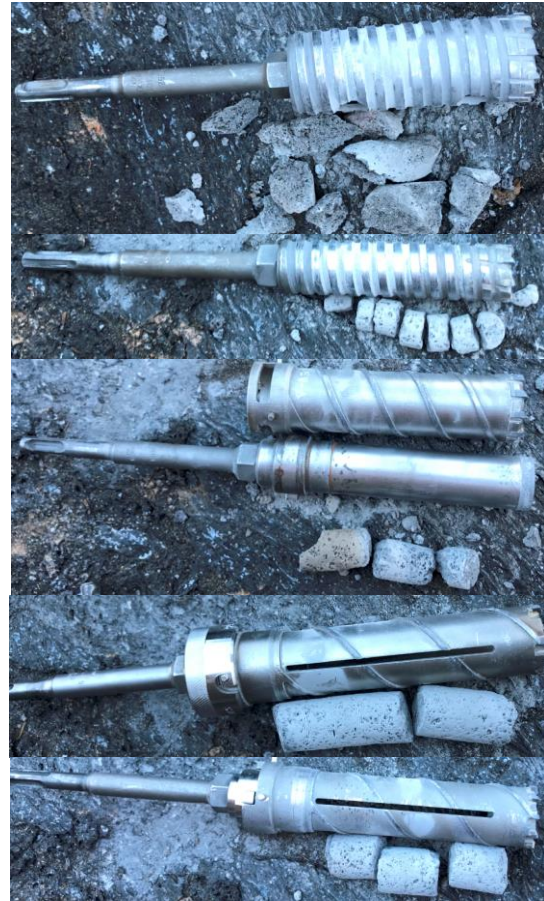
Figure 4. Coring bits tested in lava flows and captured cores. From top to bottom: A, B, C, D, and E.
