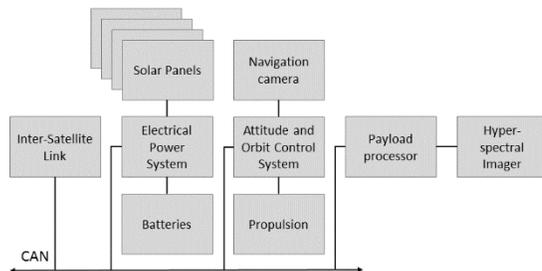
ASPECT high-level system block diagram.
