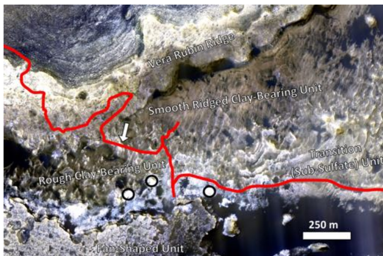
Figure 2: Color HiRISE of the clay-bearing unit along the MSL traverse. Several units of interest are labeled. The red line is the proposed Mount Sharp Ascent Route. The white arrow shows the location where the rover is planned to descend from Vera Rubin Ridge into the clay-bearing unit. The black circles show the location of several light toned mounds.
