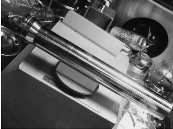
Figure 1. The CSVC (stored in the a vacuum container) used during the Apollo 17 mission had a length of 41 cm, an outer diameter of 6.1 cm and a weight of 493 g.
