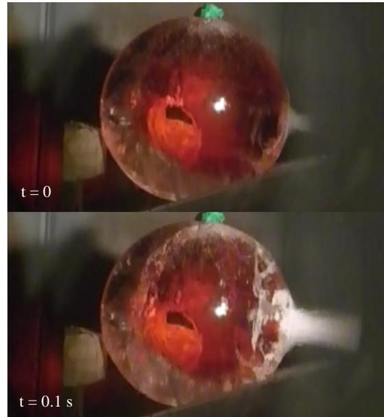
Figure 1: Still from video of  $1.97 \text{ km s}^{-1}$  impact showing the point of impact ( $t = 0$ ) where fractures have yet to form and  $t = 0.1 \text{ s}$  where the circular and radial fractures have formed. The red interior is the result of dying the internal water with food coloring.
