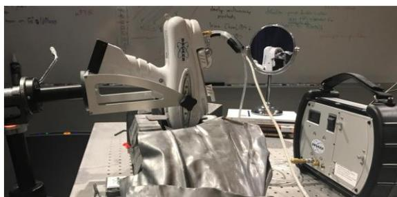
**Figure 1.** Lab benchtop setup for Tracer III-SD with vacuum at right.
