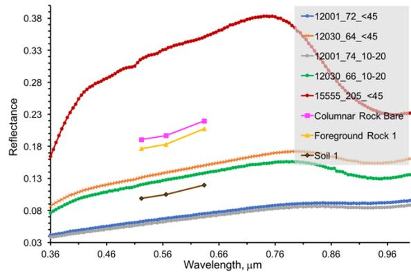
**Fig. 3.** Reflectance spectra for returned lunar samples (RELAB), with average 3-color spectra extracted from the image ROIs shown in Fig. 1A.
