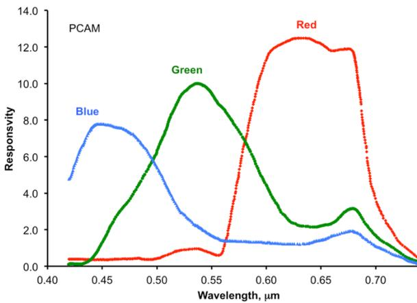
**Fig. 2.** Responsivity of the three PCAM color channels [4].
