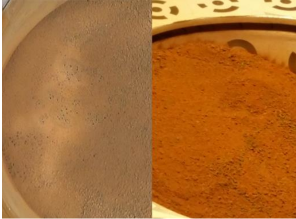
Fig. 2. Gas entrainment features. (Left) Pitting due to sublimation of CO 2 ice buried by deposition. JSC Mars-1 initially near angle of repose. (Right) Fan-shaped deposits on box sides due to rapid escape of subsurface CO 2 gas. JSC Mars-1 at 20° initial slope.
