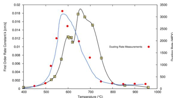
**Figure 2.** CO loss rate compared to the rate of “metal dusting” reactions producing metal carbides plus  $\text{CO}_2$  [11].
