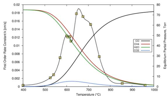
**Figure 1.** CO loss rate (yellow squares) is compared to the equilibrium fraction of CO (black line),  $\text{CH}_4$  (red),  $\text{H}_2\text{O}$  (green) &  $\text{CO}_2$  (blue) in the same gas mixture as a function of temperature.
