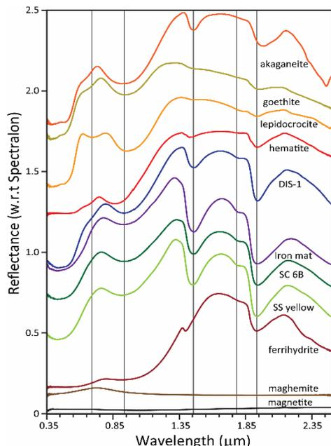
**Figure 2.** VNIR spectra of biogenic Fe(III) samples with nanophase FeOx for reference. Vertical lines mark prominent absorptions for biogenic samples.
