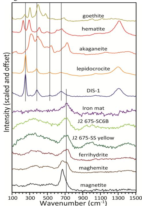
**Figure 3.** Raman spectra of biogenic Fe(III) samples with nanophase FeOx for reference. Vertical lines mark prominent absorptions for biogenic samples.
