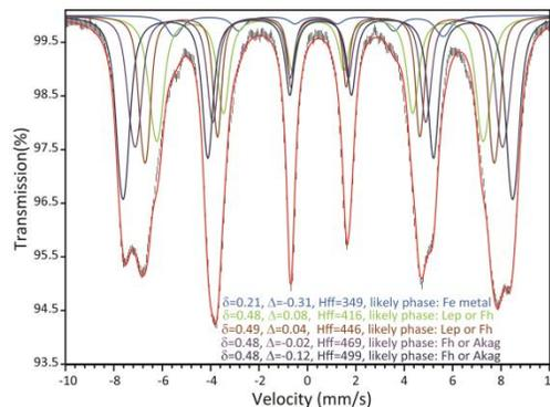
**Figure 4.** Mössbauer spectrum and fit of DIS-1 at 4K. Mössbauer fit parameters and likely phases color coded by distribution. Center shift ( $\delta$ ) and quadrupole splitting ( $\Delta$ ) are in mm/s and hyperfine field (Hff) is in kOe.
