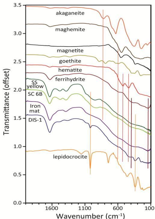
**Figure 1.** FTIR spectra of biogenic Fe(III) samples with nanophase FeOx for reference. Vertical lines mark absorptions of references and are color-coded by mineral.
