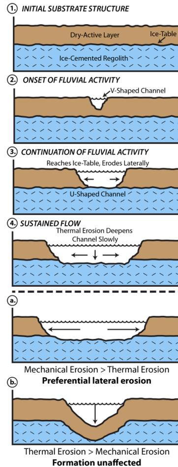
**Figure 1.** Conceptual model for channel evolution and valley network formation under cold and icy conditions [8]. The fluvial substrate is comprised of an ice-free dry active layer and ice-cemented regolith, with the interface between them being the ice-table [9].
