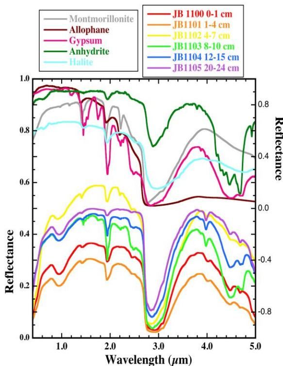
**Figure 2.** Reflectance spectra of six samples from the VXE-6 pond soil pit compared to spectra of montmorillonite, allophane, gypsum, anhydrite, and halite.
