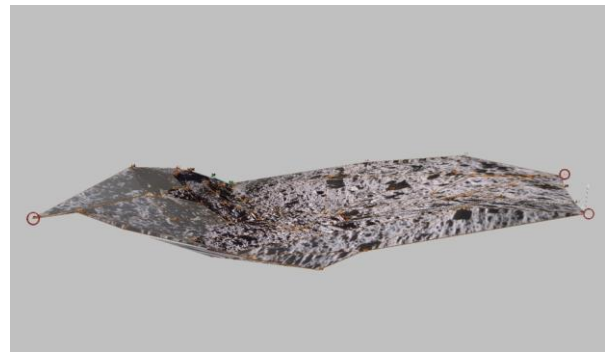
Fig. 2. Perspective view of the 70019 crater determined from the TIN triangulated by the iWP program.
