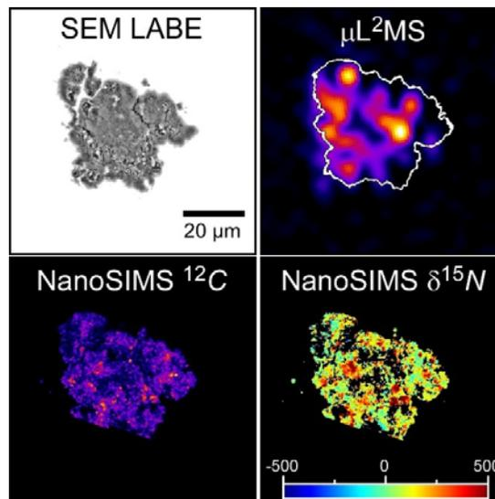
Fig 2. SEM imaging added for contextual observation of QUE99177\_NN2\_S3.  $\mu\text{L}^2\text{MS}$  image map showing spatial distribution with comparative NanoSIMS elemental C map with a  $\delta^{15}\text{N}$  map.
