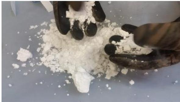
**Figure 1.** CO<sub>2</sub> “snow” made at JSC using bottled LCO<sub>2</sub> and commercial off-the-shelf hardware.
