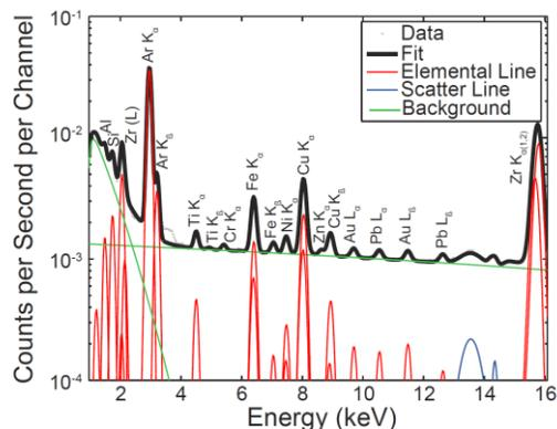
**Figure 2:** Least-squares fit of MER-B atmospheric spectra totaling 1614.5 hours in duration. With the exception of the Ar K<sub>α</sub> and K<sub>β</sub> peaks, all elemental signals originate from the APXS instrument.
