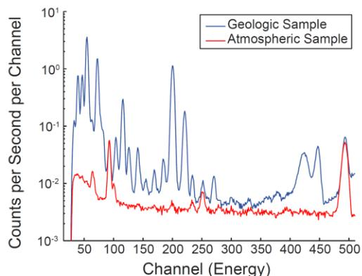
**Figure 1:** Comparison of MER-B spectra from a solid sample (blue, 11.5h duration) and atmospheric sample (red, 16h duration). The Ar K<sub>α</sub> peak is situated around channel 100.
