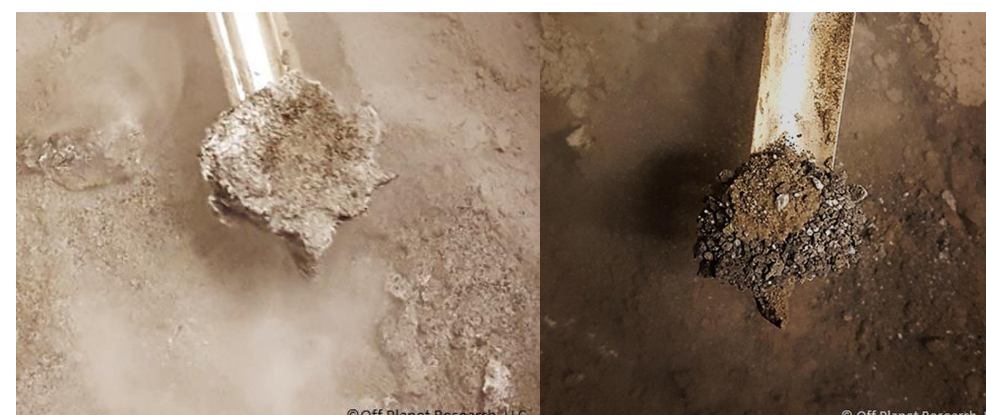
Simulated lunar ice made by OPR in Feb 2018. The images show the frozen gas components in Highland (left) and Mare (right) regolith simulants before the addition of water and methanol.
