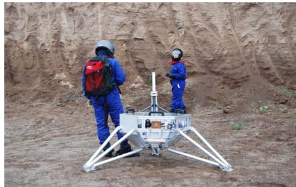
Figure 1, Two astronauts and the ILEWG ExoGeoLab lander during an analogue Moon EVA.
