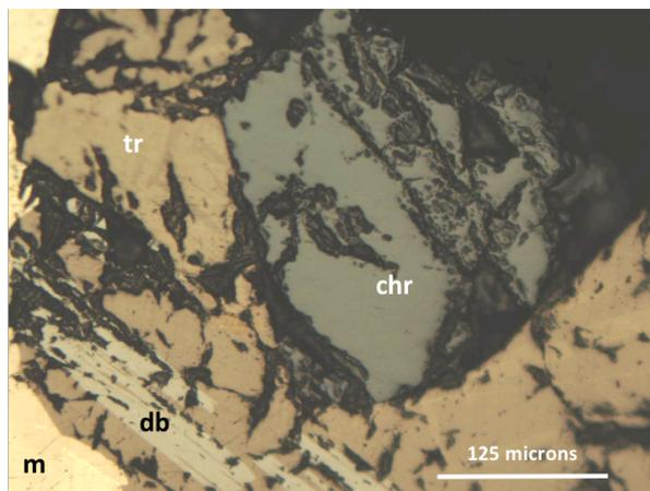
**Figure 1.** Chromite (chr) grain in Warburton Range in a matrix of troilite (tr), daubréelite (db) and metal (m).
