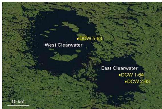
**Figure 1.** Location of drill cores at East and West Clearwater. DCW 1-64 penetrated shocked country rock in the central uplift at East [7], while DCW 2-63 drilled into the melt sheet [4]. DCW 5-63 at West Clearwater encountered melt-rich breccias [4]. Base image is Landsat scene LC80180212015250LGN00.
