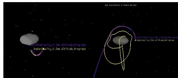
Fig 2: Prograde and retrograde satellites with 0.5km semi-major axis
