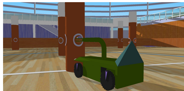
Figure 2: Pre-simulated full controllable robot and field of competition 2016 (any target can be simulated e.g. a sports hall which is the place of the contest)
