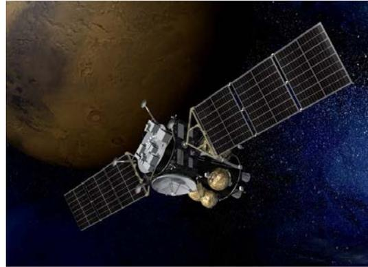
Figure 1: An example of MMX spacecraft design. Launch mass of 3400kg is composed from three stages system with return module, exploration module and propulsion module. Nominal mission duration is 5 years.
