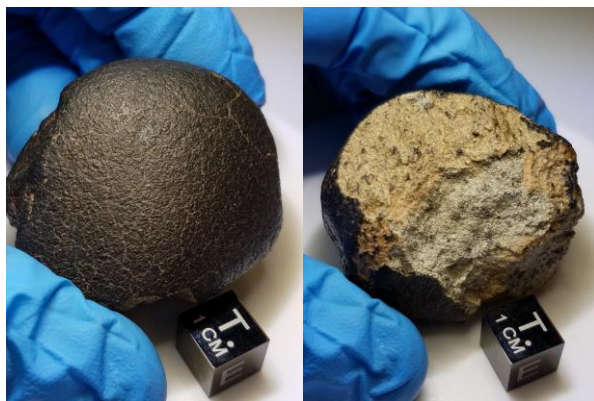
Fig. 1 NWA 11042 single stone, left shows fusion crust, right shows pale green fresh broken surface, small dark patches are shock melt pockets.
