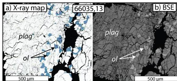
**Fig. 1:** Representative combined element X-ray map (a) and BSE image (b) of an FAN clast from regolith breccia 66035,13. White represents plagioclase and blue olivine.
