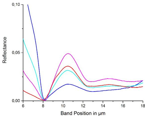
**Fig.2a:** FTIR spectrum of glass with the average composition of the lunar highlands [8].
