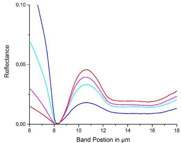
**Fig.2b:** FTIR spectrum of glass with the average chemical composition of the lunar maria [8]. It is dominated by a single RB band typical for glass.
