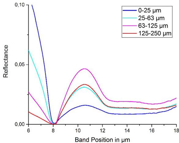
**Fig.1:** FTIR spectrum of glass based on chemical composition averaged from analyses of the surface of Venus determined by the Venera and Vega missions [7].
