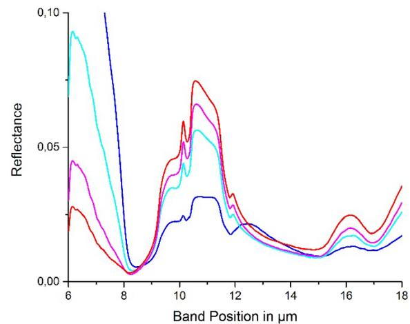
**Fig.2c:** FTIR spectrum of recrystallized glass with the chemical composition of the bulk silicate Moon [9], dominated by crystalline olivine features [10].
