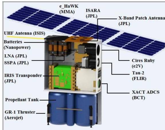
Figure 2. LOGIC spacecraft layout. The spacecraft is expected to be a 14 kg, 6U CubeSat with a visible and thermal camera, onboard green monoprop propulsion system, X-band radio and Blue Canyon XACT attitude determination and control system suite.
