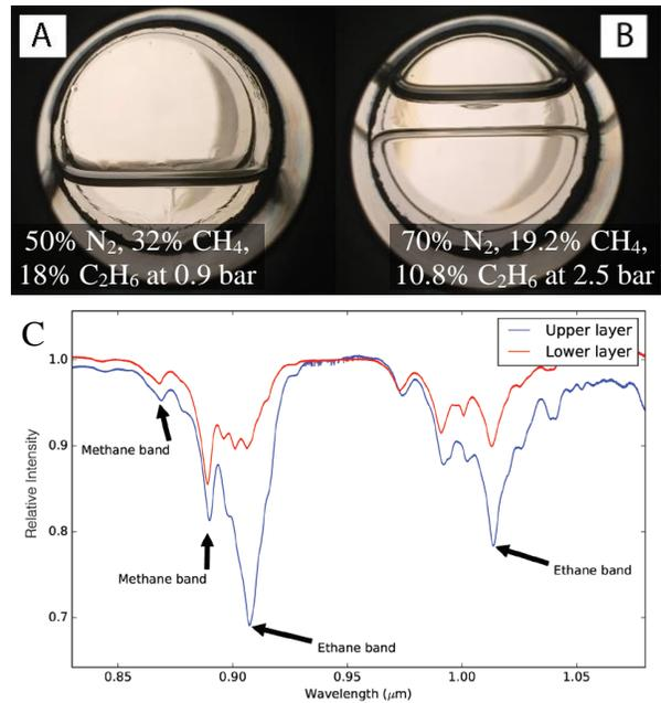
**Figure 4.** Images taken at low (A) and high (B) pressure. (C) Spectra of the top and bottom layer from experiment B.
