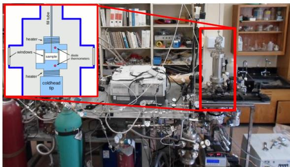
**Figure 1.** Photo of laboratory setup. Inset: Schematic of the cell.
