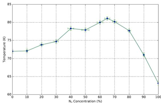
**Figure 3.** Freezing points of nitrogen-ethane-methane mixtures for varying amounts of nitrogen and a constant remainder ratio of 64% methane:36% ethane.
