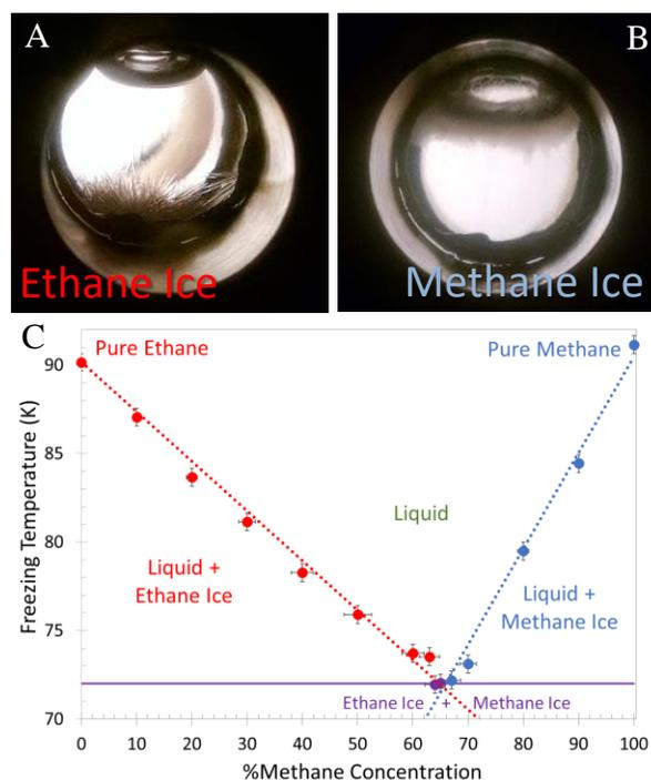
**Figure 2.** Freezing points of solutions with varying methane/ethane concentrations. (A-B) Images of mixed methane and ethane solutions at their freezing points. Ethane ice freezes first (A) when the concentration falls on the ethane liquidus (red line in C), whereas methane ice forms on the top of the solution (B) when the methane liquidus (blue line).
