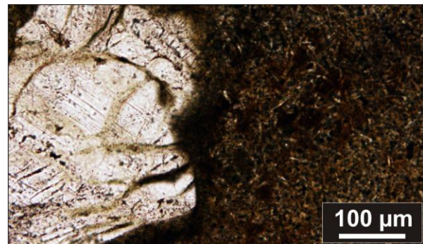
Fig. 1. Microphotograph (plane-polarized light) of an impact melt rock sample with tiny phenocryst laths (~25 \mu\text{m} ) in an aphanitic groundmass. On the left side is a partly digested shocked quartz clast. Sample M0077A_93R3_51-52 (740.9 mbsf).
