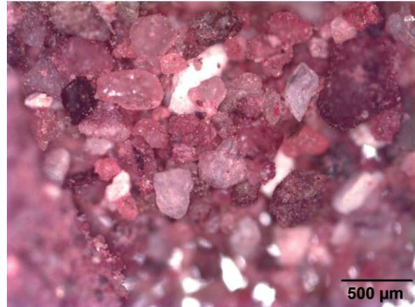
Figure 2.: The microscopy photo from 1 cm depth of the last drilling area (0601). Quartz, carbonate, dark minerals and clay can be seen. The shape of the grains are variable (rounded, irregular), rough surfaces with sharp and sometimes blunt edges.
