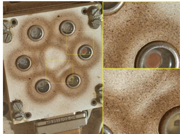
Figure 1: Sol 323 MAHLI image of the UVS, taken after the passage of the regional dust storm. Dust grains sticking to the magnetic rings with different albedos and colours are seen.
