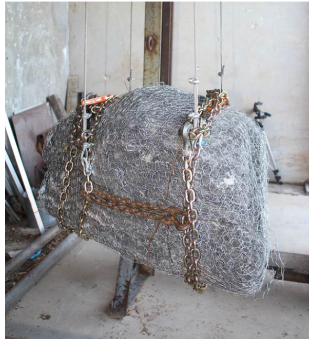
Figure 1. Ballistic pendulum suspension setup for pumice rock shots.
