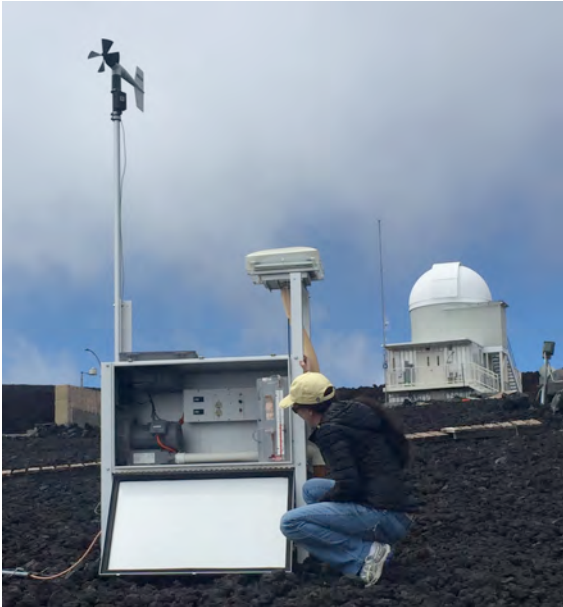
Figure 3: High-volume air sampler with anemometer at Mauna Loa Observatory.
