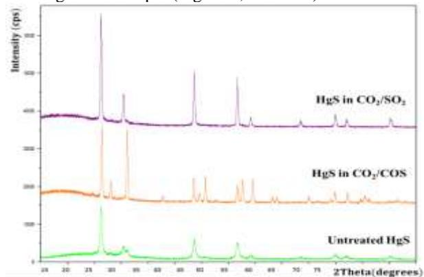
**Figure 1:** XRD results of the metacinnabar experiments. Untreated metacinnabar is graphed at the bottom, followed by metacinnabar heated in  $\text{CO}_2/\text{COS}$ , followed by metacinnabar heated in  $\text{CO}_2/\text{SO}_2$ .
