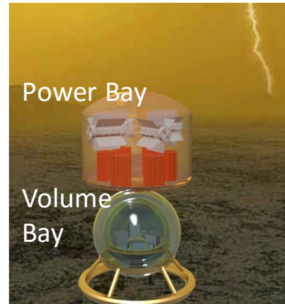
Figure 1. Proposed Venus Lander Configuration (background apadted from [5])
