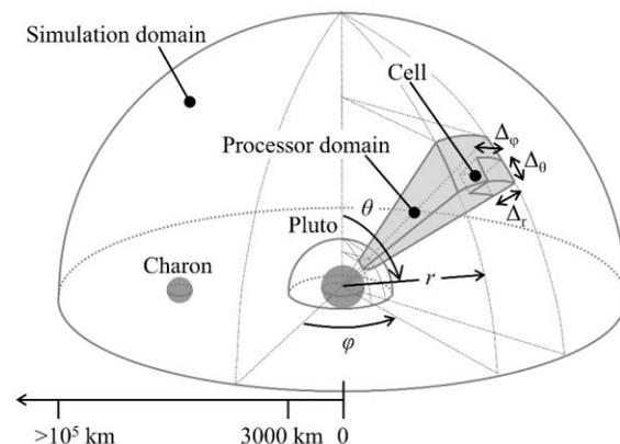
**Figure 1.** Shape and extent of a hemispherically-symmetric simulation domain. (Cell size not to scale.)
