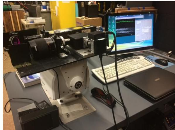
Figure 1: Compact remote Raman+LIBS+Fluorescence system (CRRFLS) mounted on a movable pan/tilt scanner.
