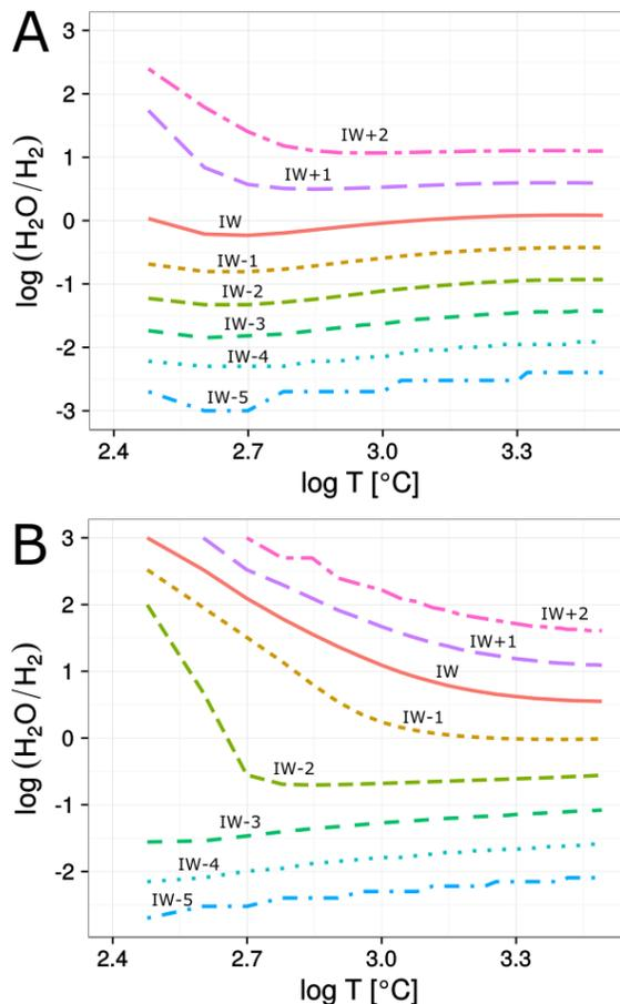
**Figure 1.**  $\log_{10}(\text{H}_2\text{O}/\text{H}_2)$  as a function of ( $\log_{10}$ ) temperature at specified *f*O<sub>2</sub> conditions, calculated for A) 1 kbar pressure, and B) 10 kbar.
