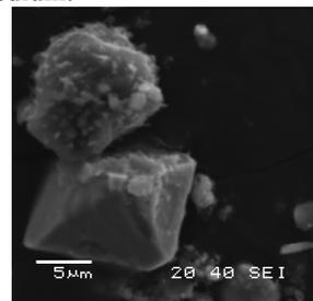
**Figure 1** SEM image (15 kV) of a lyophilized snow alga (top) covered in particles, likely both bacteria and minerals, and magnetite (bottom) collected from Mount Anderson Ridge, CA
